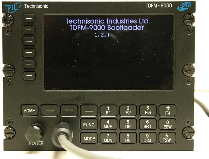
FIGURE 9: The Bootloader Screen
