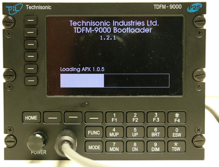
FIGURE 14: Radio Progress Screen
