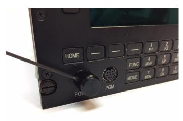
• Remove the 6 black screws from the plastic front panel:
