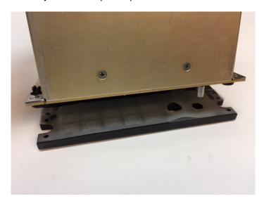
• Remove the metal and fiber spacers from the panel:
