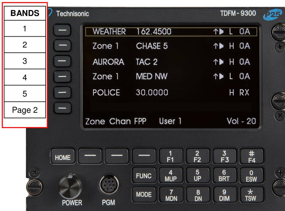
FIGURE 3: TDFM-9300 Band Display Orientation
